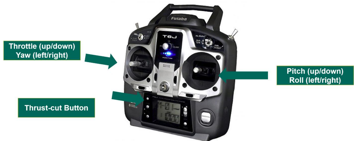
Figure 23: Controller and its controls
